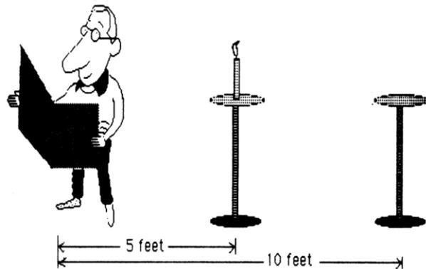
A man is reading a newspaper by the light of a single candle five feet away. There's your unit distance. Make that a relative distance equal to one. Indicate the number of candles necessary to light up the paper to the same brightness if the table were moved to a distance of ten feet. In other words that would be a relative distance of two units. We are doubling the distance.
